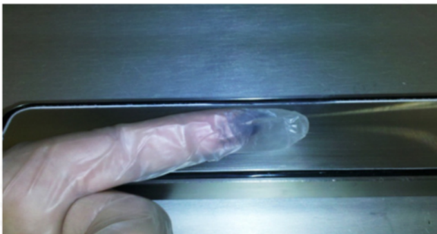
Competitive FFKM with heavy white residue build-up
